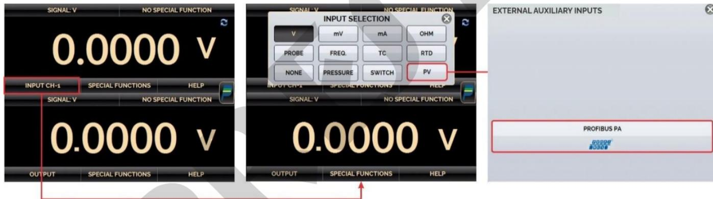
Fig. 58 - Profibus® input selection
