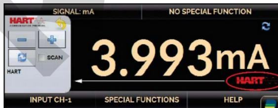
Fig. 49 - Quick Hart® Adjustment with Reference
